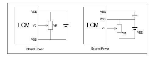
$V_{DD^{\sim}}V_0\text{: LCD Driving voltage}$
